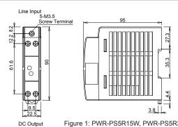
Figure 1: PWR-PS5R15W, PWR-PS5R30W Physical Dimensions (Consult factory for other model drawings)
