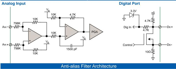
The DI-4108 employs an anti-alias filter per analog channel with automatic corner frequency selection. The filter is a CIC (cascaded integrator comb) type that applies as many as 512 samples per channel to calculate filter results in real time. Filter response is optimized when sampling frequency is set to ten times the highest frequency of interest.
