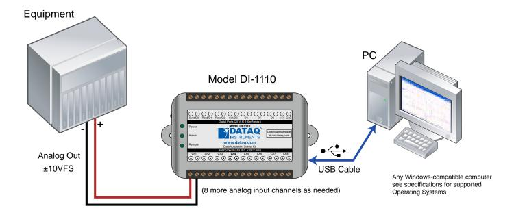
Examples of "Equipment" above include gas chromatographs, liquid chromatographs, spectrometers, bio-amplifiers\*, etc.
